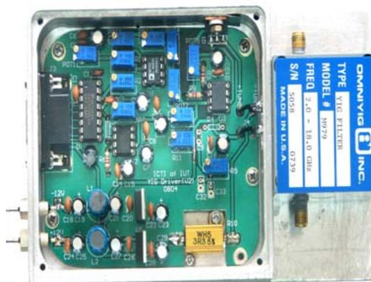
Fig. 19. Photograph of YIG filter and driver
