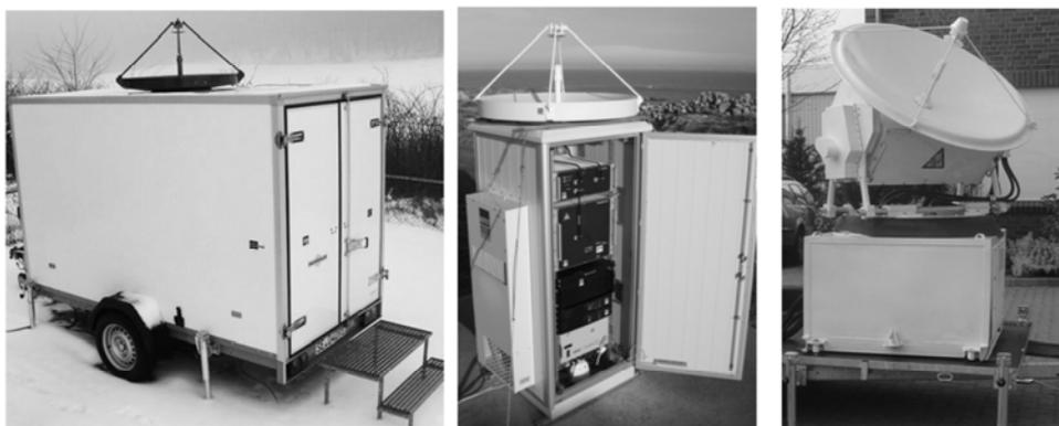
Fig. 2. Ka band magnetron based meteorological radars.
