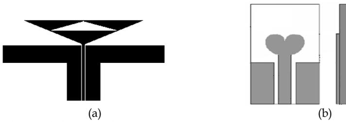
Fig. 10. Printed CPW-fed monopole antennas<sup>[18, 19]</sup>
