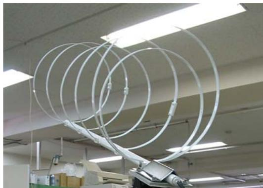
Photo 2. Right-hand Circularly Polarized Ring Loop Antenna
